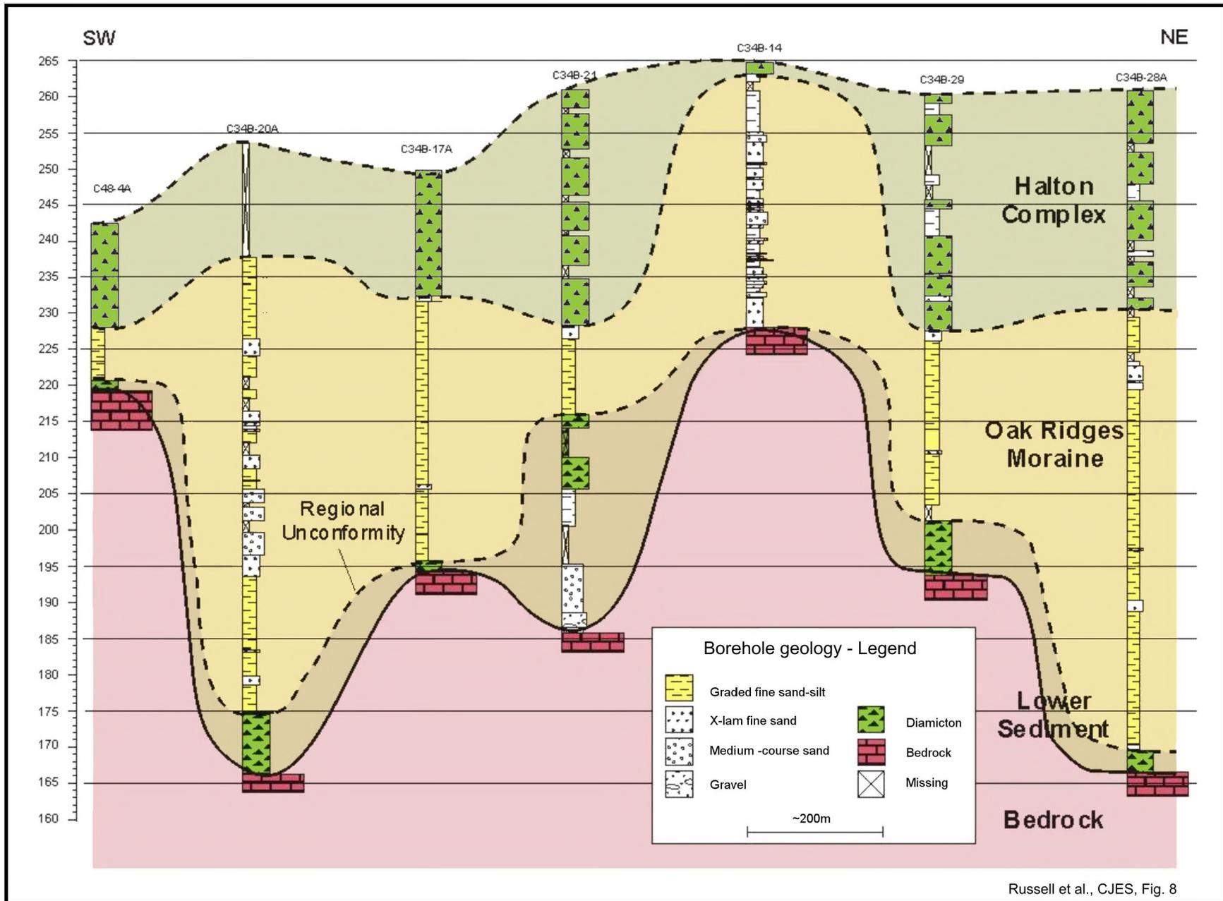
**Figure 6.** Simplified geological cross-section of the area southwest of Bolton, based on selected borehole geologic logs from the IWA investigation site (re-interpreted by Russell (2001) after Blair (1994)).
