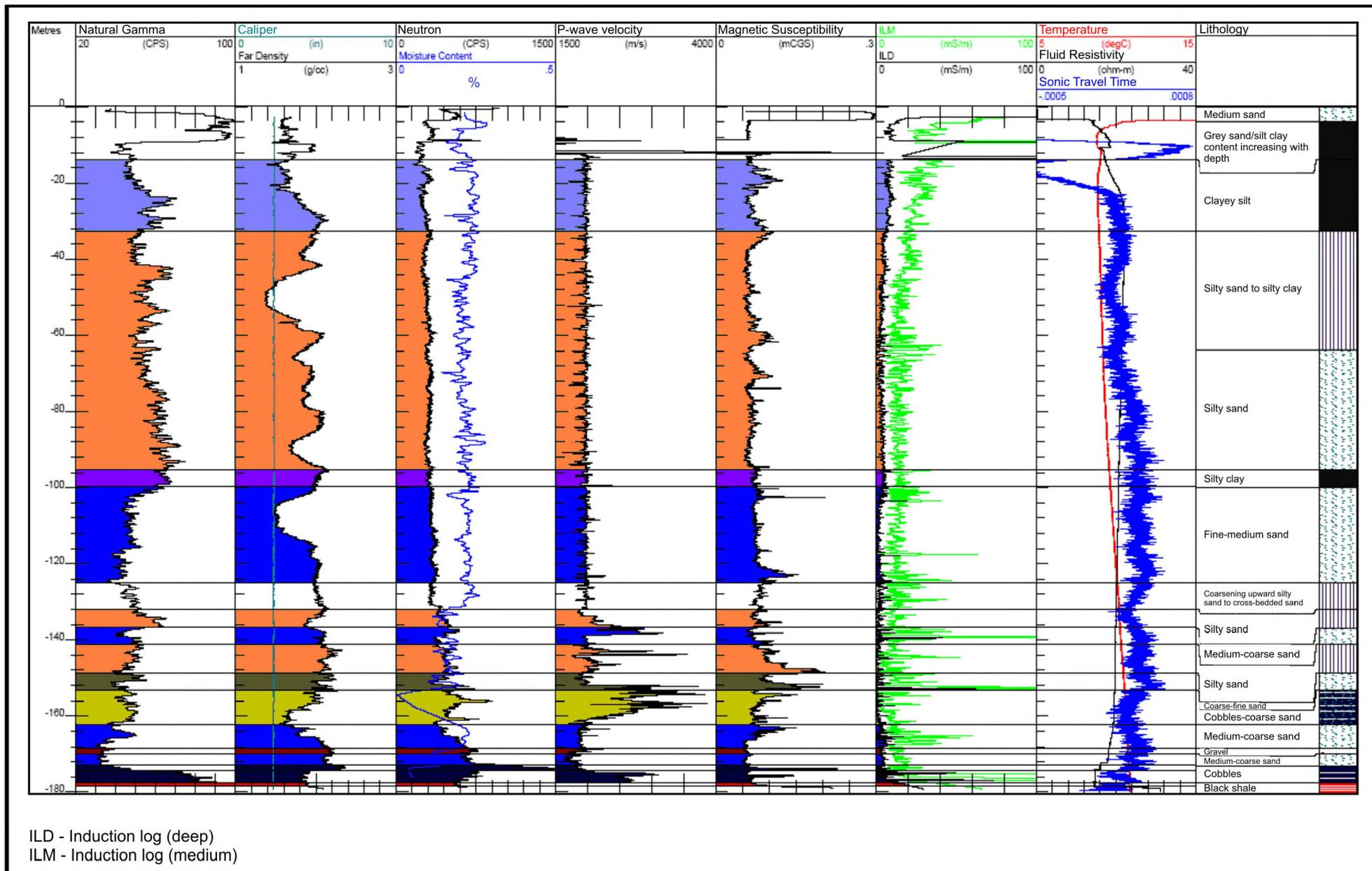
**Figure 9.** Downhole geophysical logs for borehole CAMC/YPDT-Heart Lake Road. Explanation of units of measure: CPS = counts per second; in = inches; g/cc = grams per cubic centimetre; m/s = metres per second; mCGS = millicentimetres per gram per second; mS/m = milliseconds per metre; degC = degrees Celcius; ohm-m = ohms per metre.
